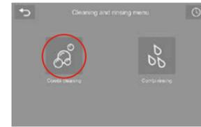
Press the COMBI-CLEANING button to start cleaning.
