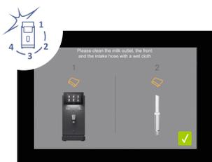
Clean the milk outlet according to the hygiene concept.
