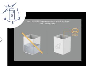
Then place a milk cleaning tablet in the empty cleaning container.
