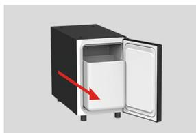
Open the refrigerator door and remove the milk container.
