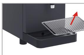
Remove the drip grid from the residual water tray and clean it.
