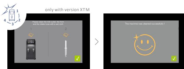
Clean the milk outlet according to the hygiene concept.
