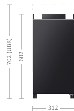
10l Cooler R10 / R10 UBR (under-counter) 30 kg | 0.09 kW 2)
